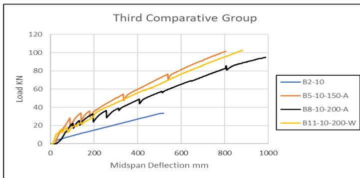
**Fig.7:** Load -midspan deflection for third comparative group beams with Ø 10.
