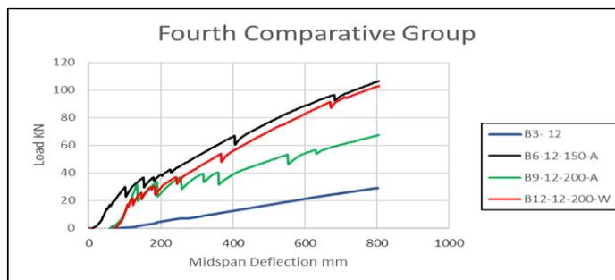
**Fig.8:** Load -Midspan deflection for fourth comparative group beams with Ø 12.
