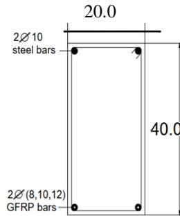
**Fig. 1:** Beam Cross-Sectional Area and Reinforcement Detailing
