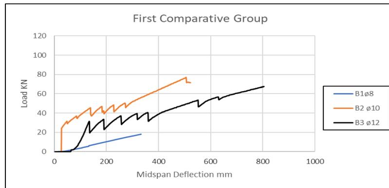
**Fig. 5:** Load -midspan deflection for first comparative group.
