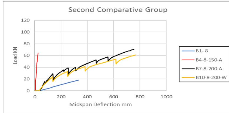
Fig.6: Load -midspan deflection for beams with Ø 8.
