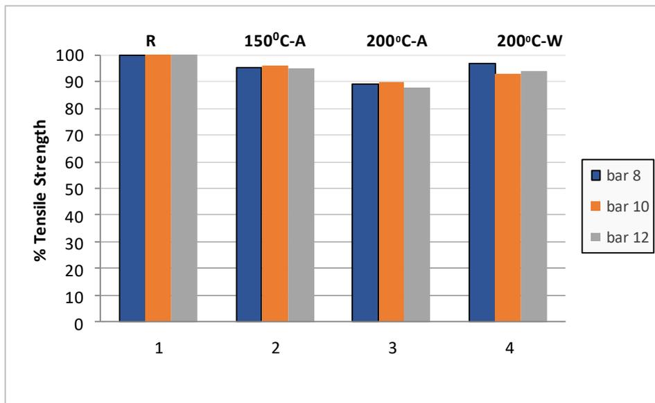
**Fig: 4** Percentage Ratios for Bars Tensile Test Results.
