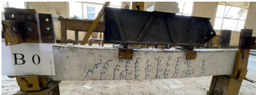
Figure 3.6: Failure Mode and Crack Pattern of Control Beam
