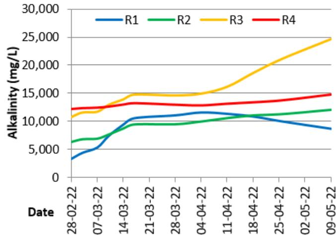
Figure 4: The Bioreactors Initial Alkalinity.
