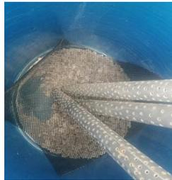
Figure 1(c): Gravel Layer with the Two LDPE Covering Sheets.
