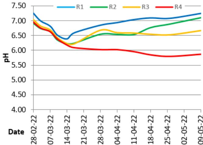
Figure 3: The Bioreactors Initial pH.
