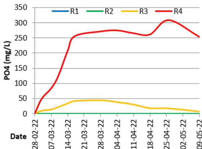
Figure 10: The Bioreactors Initial Phosphate Concentrations.
