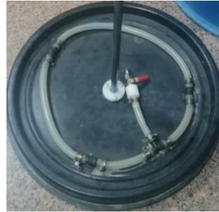
Figure 1(d): The Gas Collection System
