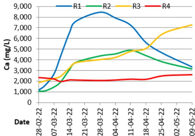
Figure 5: The Bioreactors Initial Calcium Concentrations.
