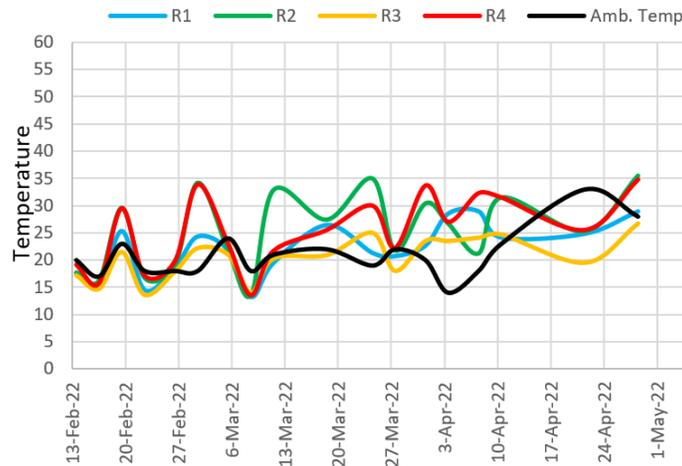
Figure 2: The Bioreactors Temperature vs. the Ambient Temperature.
