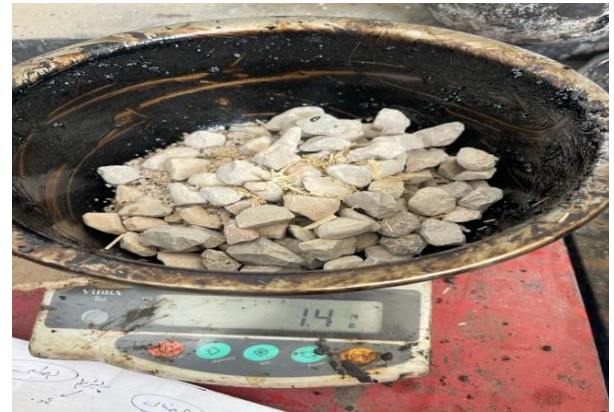
Figure 14: Flax- shives fibers with aggregate
