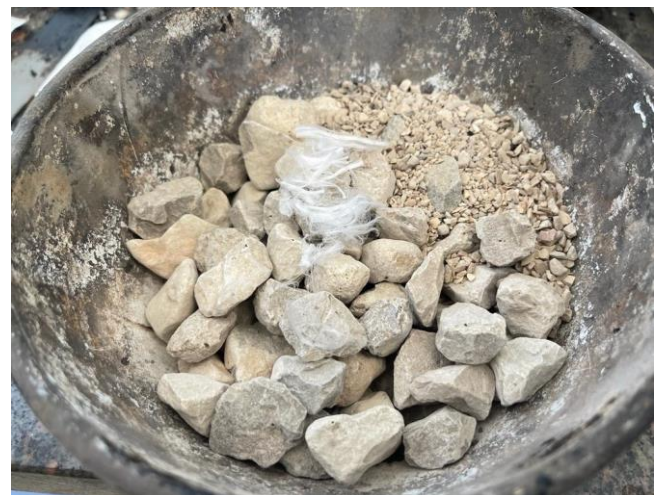
Figure 10: Polypropylene fibers with aggregate.
