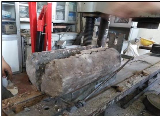
Figure 6. Splitting tensile strength test
