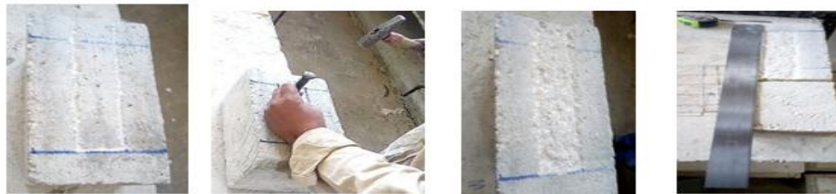
a. Marking line on prism b. Grinding and grinding tools c. Surface cleaning with the brush and hover
