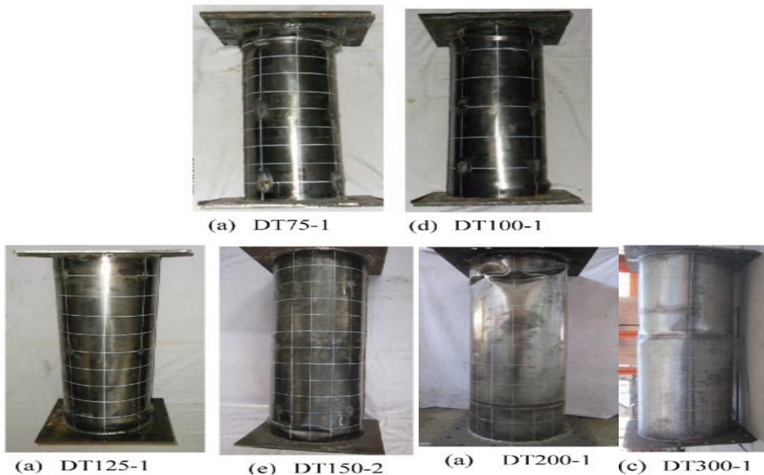
Figure 1. Failure mode of specimen \lambda_s = 60.5 to \lambda_s = 242 (Lanhui Guo, Yong Liu, Hui Jiao, and Shilong 2016).
