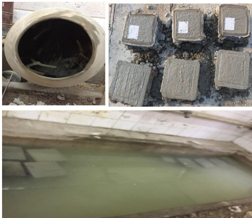
Figure 1: Mixing, Casting and Curing for Concrete Cubes Specimens.
