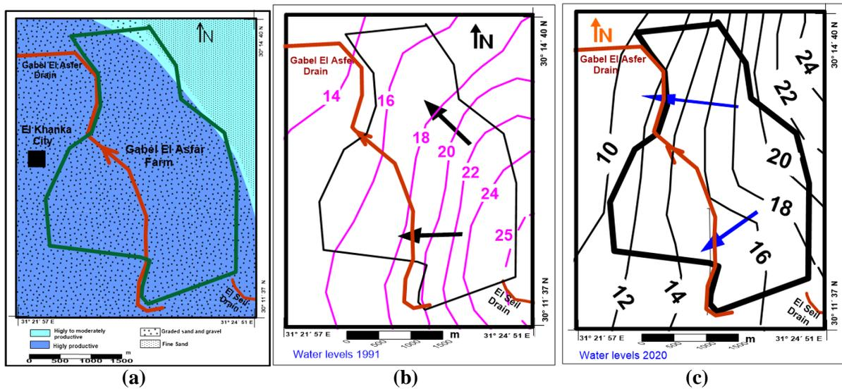
Figure 3: Aquifer System (a) and Water Levels in Gabel El Asfer Farm in 1991 (b) & in 2020 (c)
