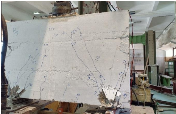
Figure 10 - Crack pattern and failure mode for specimen (B3)
