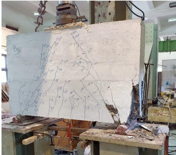
Figure 12 - Crack pattern and failure mode for specimen (B5)
