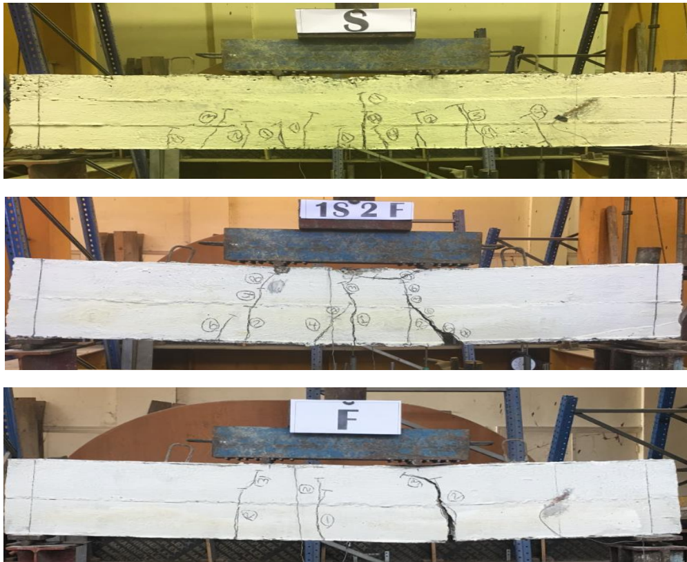
Figure (3): Crack Pattern for Tested Beams
