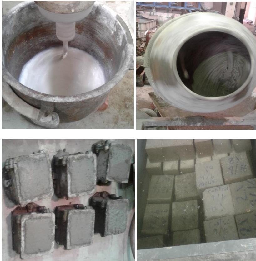
Figure 1. Mixing, Casting and Curing for Concrete Cubes Samples
