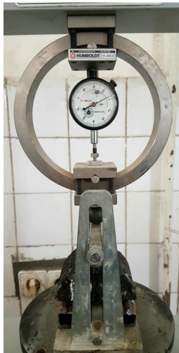
Figure 8: Three-point bending set-up
