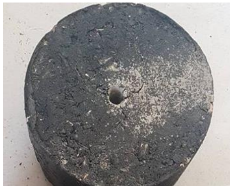
Figure 2: Marshal test specimens for microwave heating.
