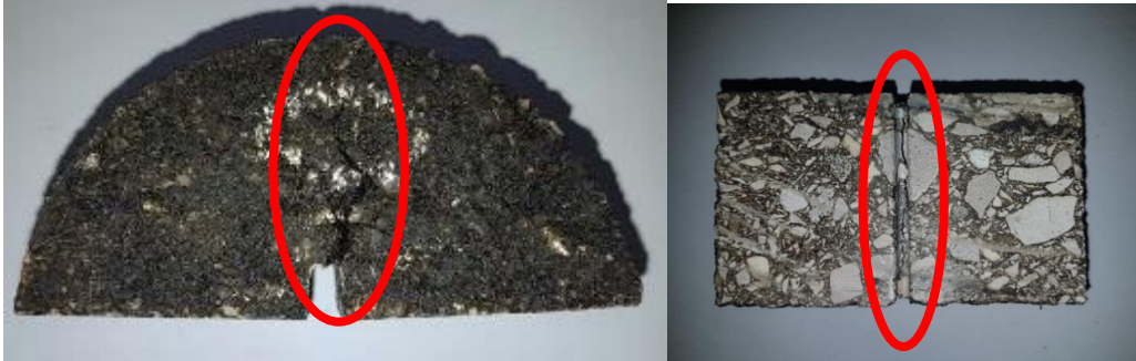
Figure 10: Cracked sample before microwave heating.
