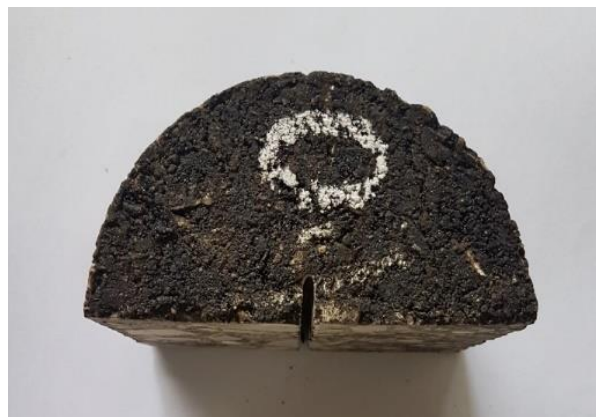
Figure 11: Cracked sample immediately after microwave heating
