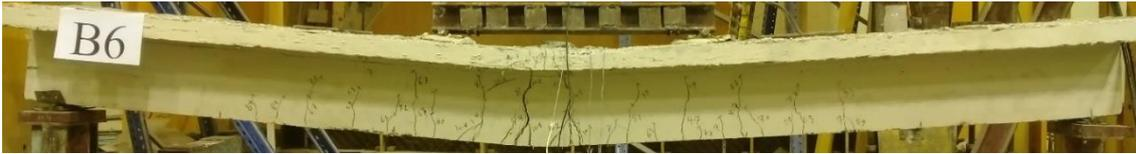
Fig. 9: Crack Pattern and Failure for Specimen B6 (LLU-0.70)
