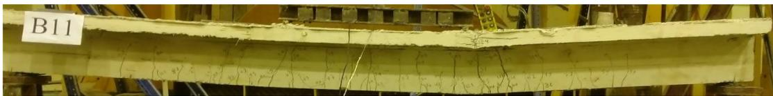
Fig. 11 :Crack Pattern and Failure for Specimen B11 (LTB-0.70)
