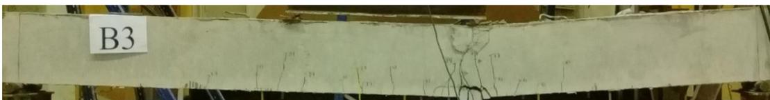
Fig. 7: Crack Pattern and Failure for Specimen B3 (LRU-0.70)
