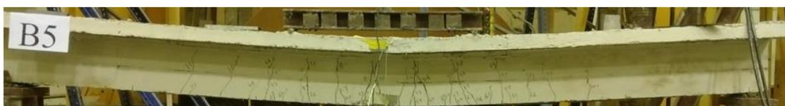
Fig. 8: Crack Pattern and Failure for Specimen B5 (LTU-0.70)
