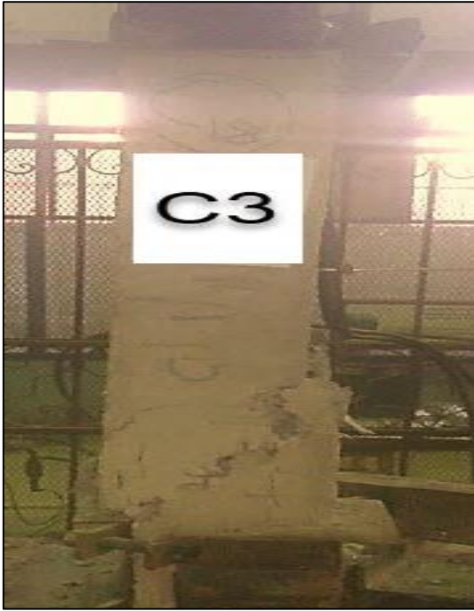
Fig. 9. Failure mode of Specimen C3
