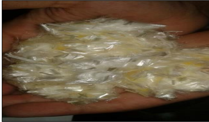
Fig. 1. Shape of polyvinyl alcohol (PVA) fibers.
