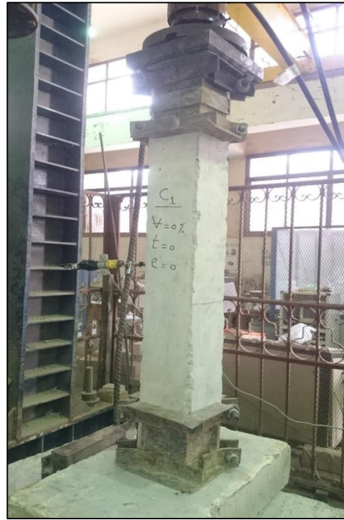
Fig. 6. Typical column during testing.
