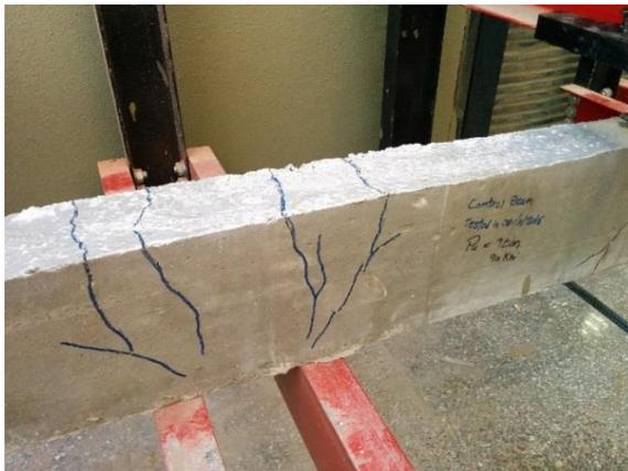
Figure 9a: Crack patterns at the beam upper surface of the beam (-ve moment)
