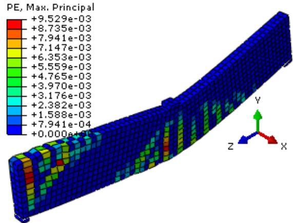
Figure 8d: Propagation of cracks at critical sections (80%  $P_u$ )
