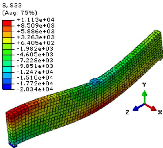
Figure 10a: S33 contours at load initiation
