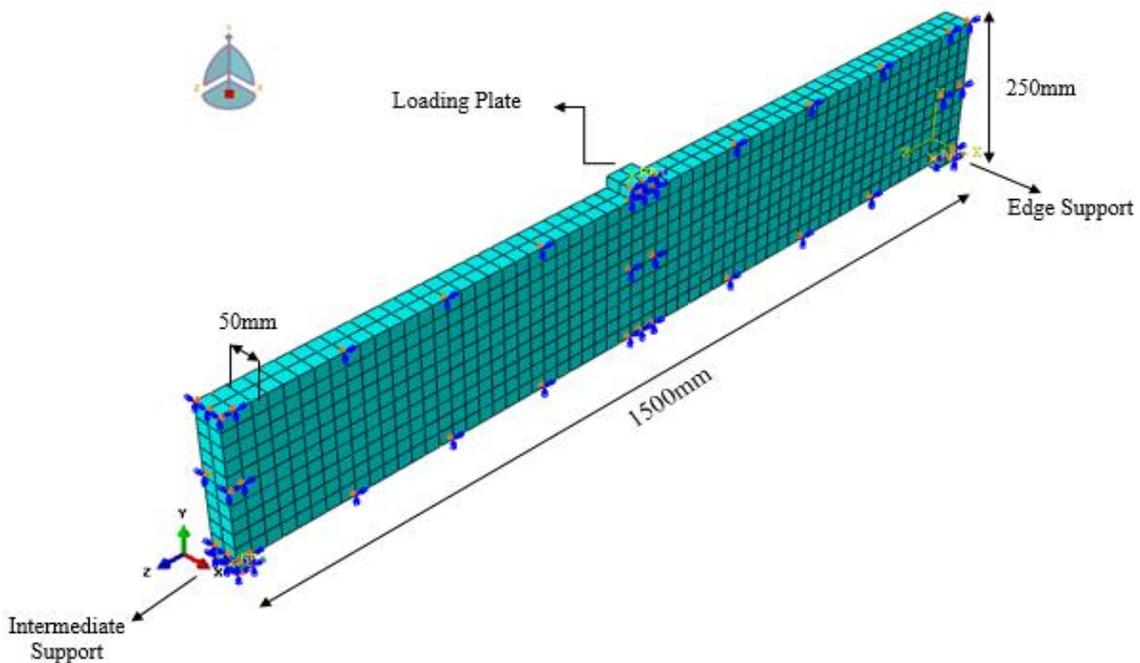
**Figure 3: Geometry, mesh, and boundary conditions of the finite element beam**
