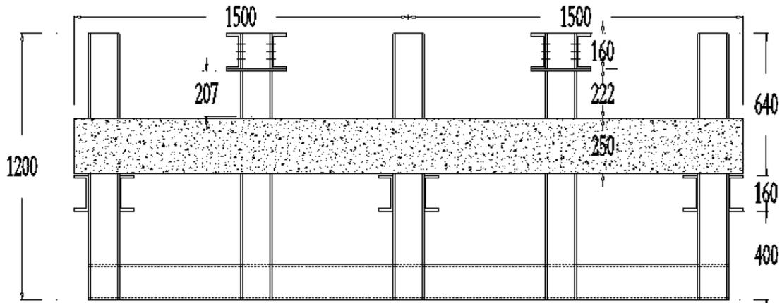
**Figure 2: Schematic drawing for a beam loaded in the loading frame, dimensions in mm**
