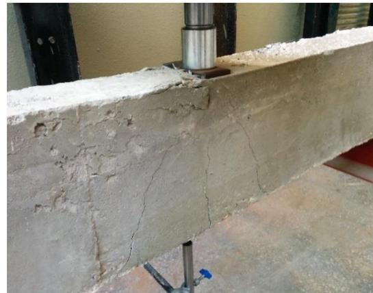
Figure 9b: Crack patterns at the lower surface at the middle of the right span (+ve moment)
