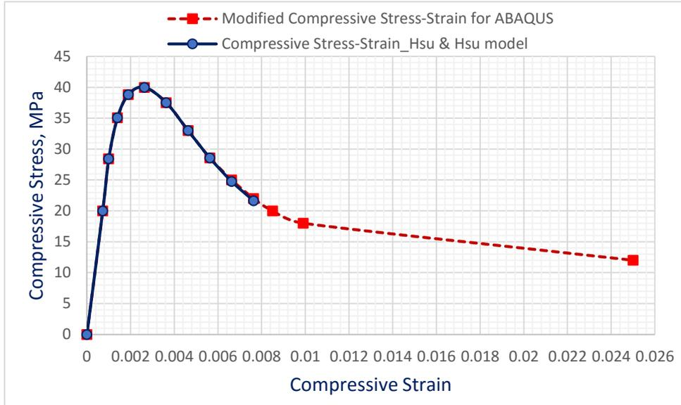
**Figure 6: Compression stress-strain relationship for concrete used for ABAQUS**
