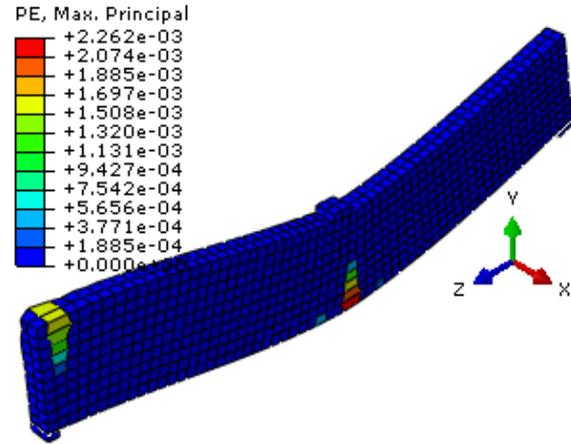
Figure 8b: Propagation of cracks at critical sections (20%  $P_u$ )
