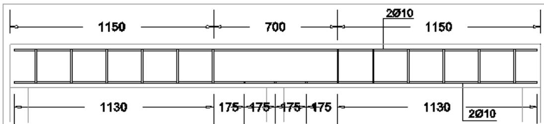
Figure 1: Beam's reinforcement detailing, dimensions in mm
