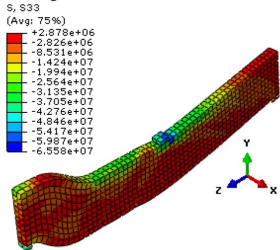
Figure 10d: S33 contours at 80%  $P_u$
