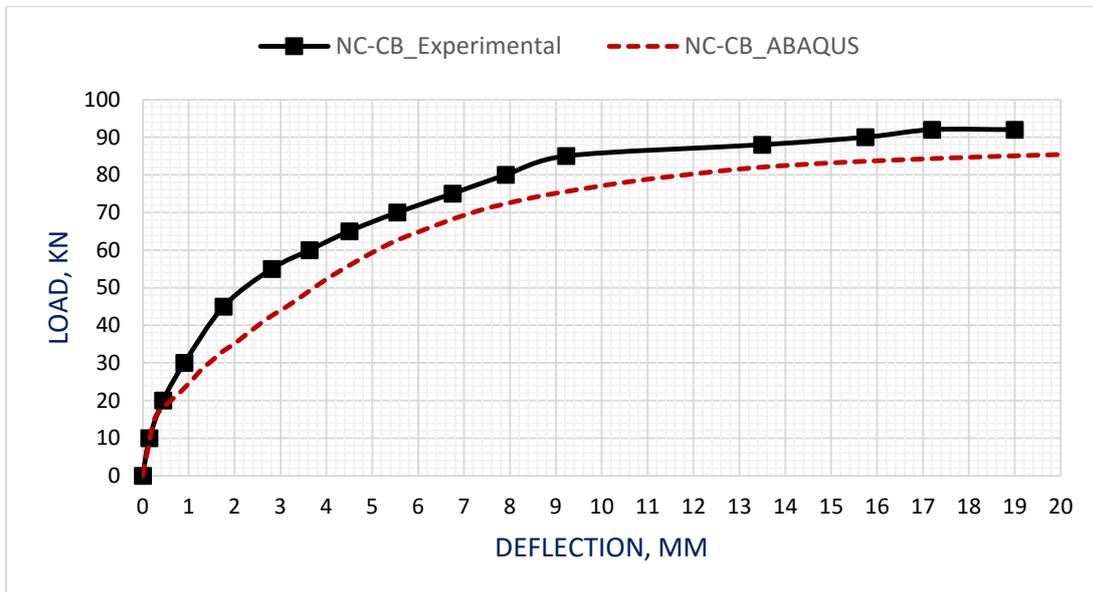
Figure 7: Load-deflection curves for the experimental Vs. the ABAQUS beam
