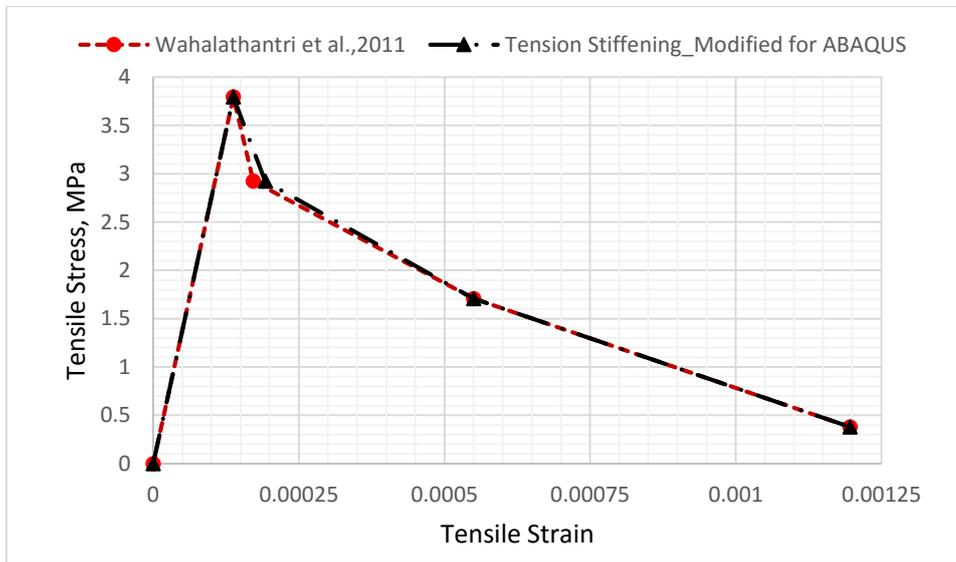
**Figure 5: Modified tension stiffening model**
