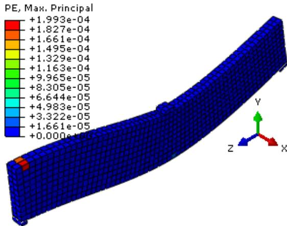
Figure 8a: Initiation of cracks at the upper face of the beam at the beginning of loading
