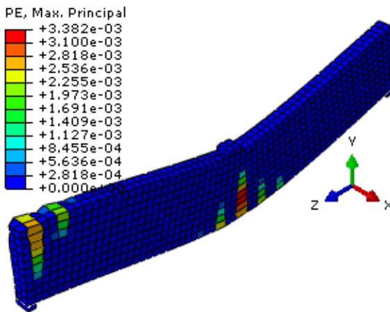
Figure 8c: Propagation of cracks at critical sections (50%  $P_u$ )
