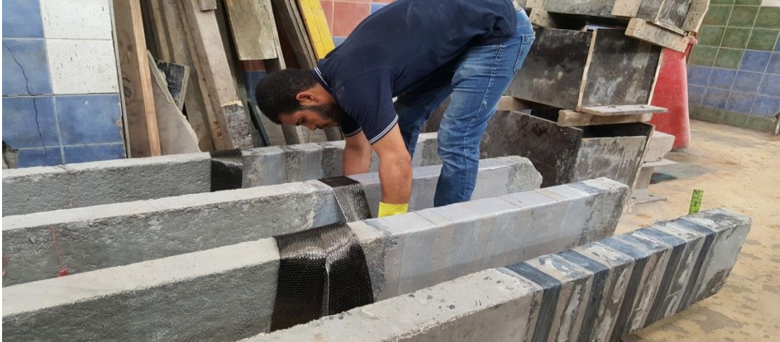
Fig. (4) shows U- wrapping shape of FRP
