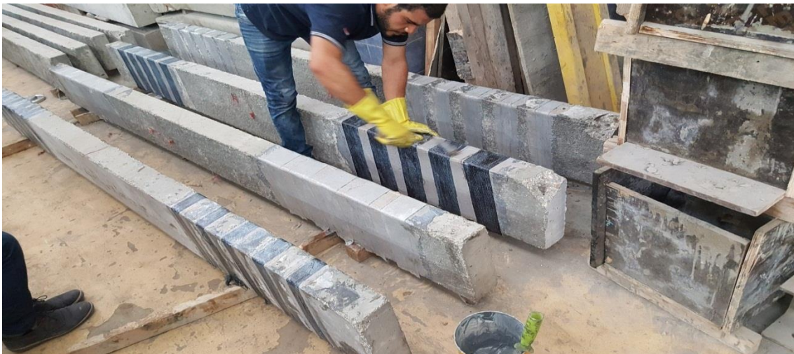
Fig. (5) shows rolling the FRP sheets
