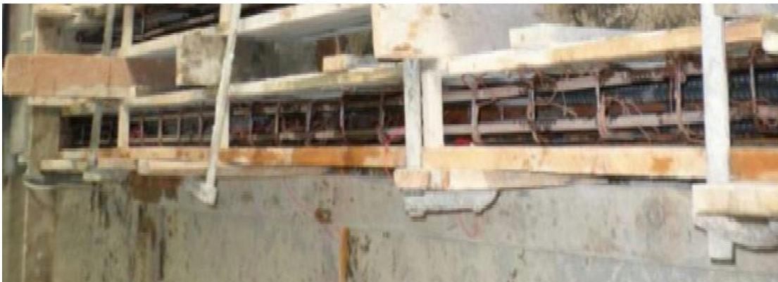
Fig (3) shows steel reinforcement of specimens in the plywood form
