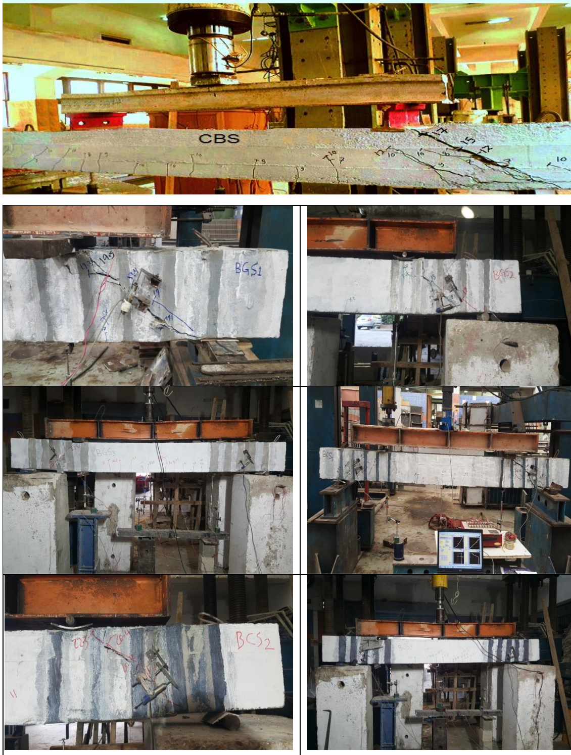
Fig. (7) shows crack pattern of beam specimens
