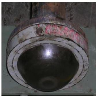
Fig. 2: Lubricated cylindrical bearing (Gao et al., 2013)
