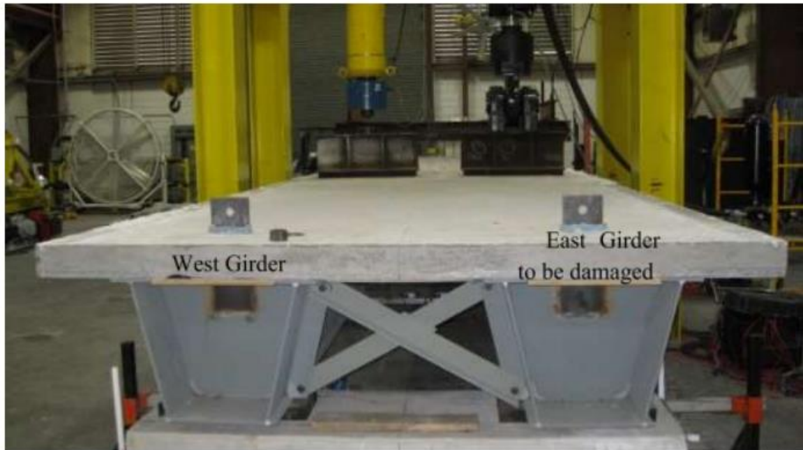
Fig .6 Specimen with complete loading setup. (Pham, 2016) 16
