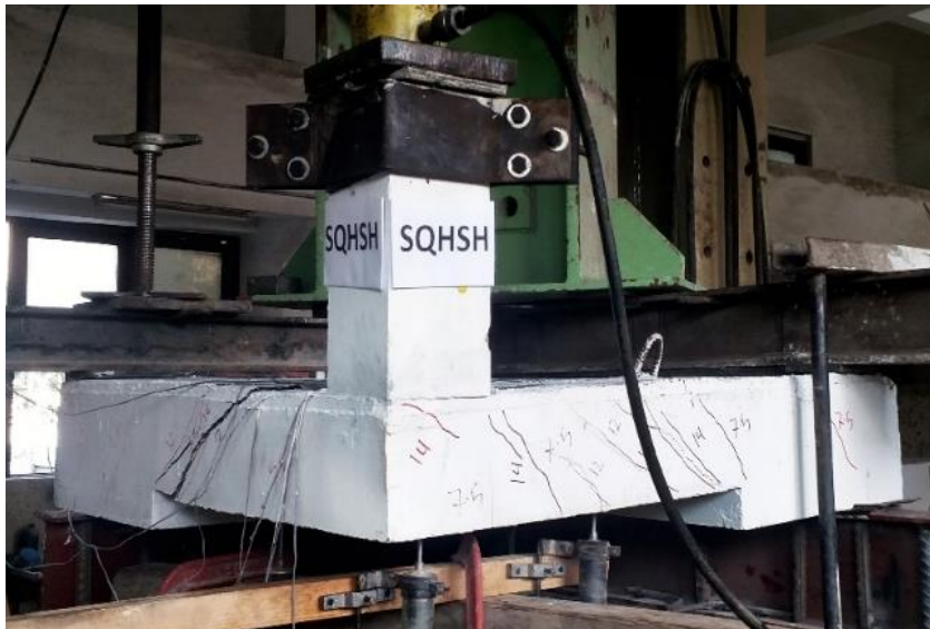
Fig. 4: punching failure for specimen (SQHSH)
