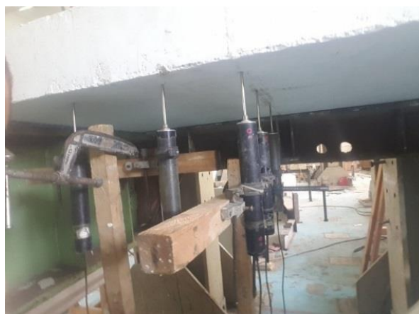
Fig.8: LVDT arrangement for specimens
