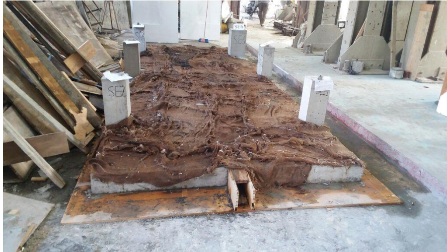
Fig.5: specimen curing by covering with wet burlap
