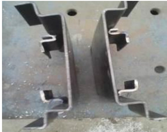
Figure (3): Partial bent up half flange for the channel (every 10 cm) (P4)
