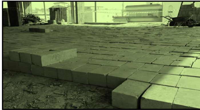
Fig. 8. Loading by Concrete Blocks uniformly distributed load
