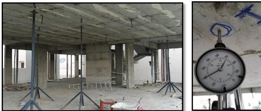
Fig. 14: Location of Dial Gauges.of S.F.R
