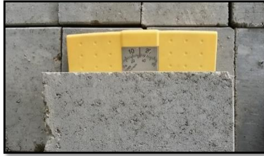
Fig.6 Weight of unit concrete block equal 15 kg/one
