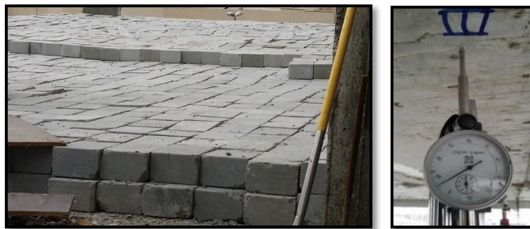
Fig. 16: Loading by Concrete Blocks uniformly distributed load
