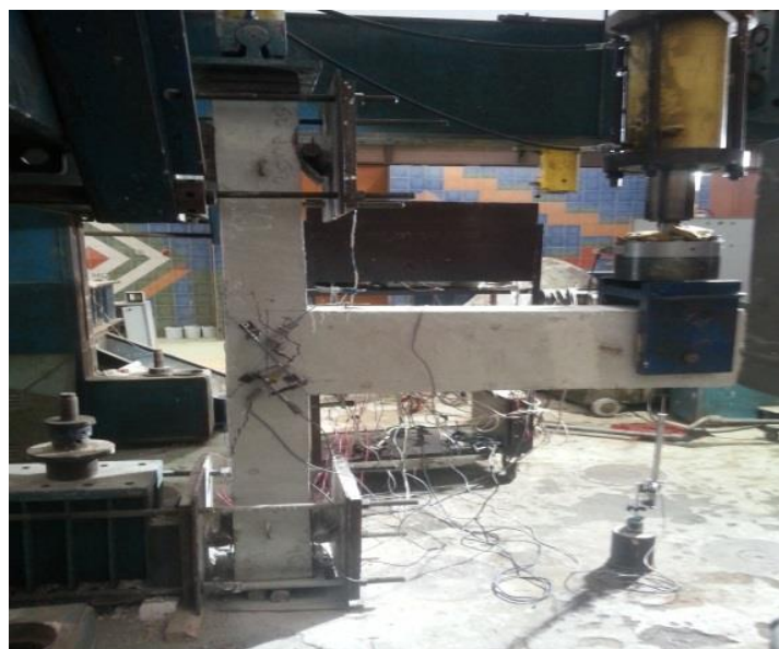
Figure 1-c: Location of LVDTs
