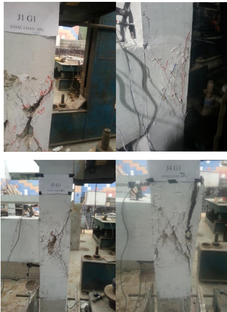
Figure 5: Crack pattern of all specimens
