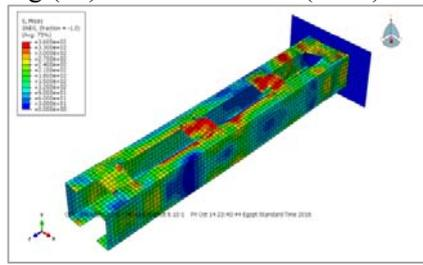
Fig (41): Failure mode of (FEM) C6
