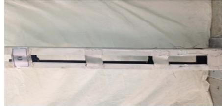
Fig. (24) Failure mode of C6 in (batten plate)
