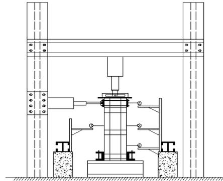
Fig. (2): Test setup and schematic view of batten steel column
