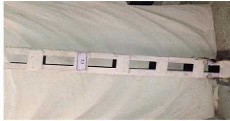
Fig. (22): Failure mode of C4 in (bottom)
