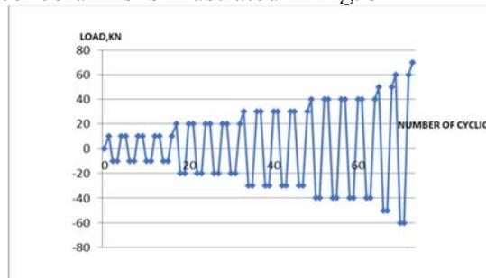
Fig. (3): Load sequence diagram
