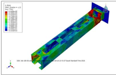
Fig (38): Failure mode of (FEM) C3
