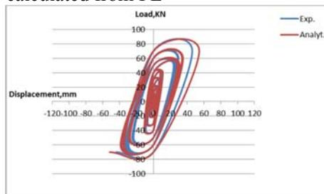
Fig. (52): Comparison between experimental hysteresis loop of column C14 and that calculated from FE.
