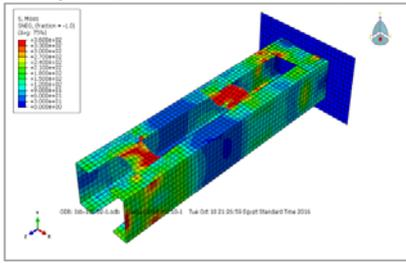
Fig (46): Failure mode of (FEM) C11
