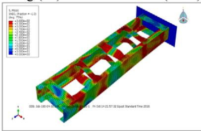
Fig (40): Failure mode of (FEM) C5
