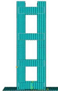
Fig (34): Meshes of batten column C12. Fig (35): Meshes of batten column C14
