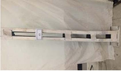
Fig. (19): Failure mode of C1 in (batten plate)
