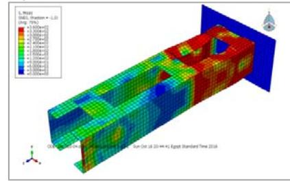
Fig (47): Failure mode of (FEM) C12
