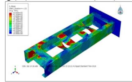
Fig (45): Failure mode of (FEM) C10
