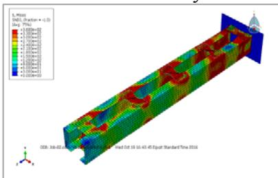
Fig (36): Failure mode of (FEM) C1
