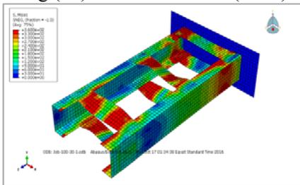
Fig (50): Failure mode of batten column C15
