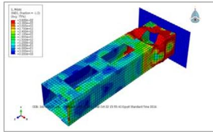
Fig (49): Failure mode of (FEM) C14
