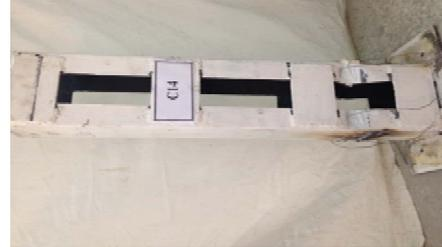
Fig. (32): Failure mode of C14 in (bottom)
