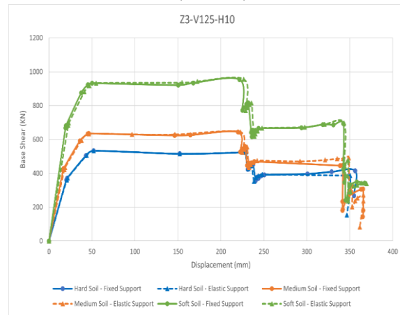
Figure (18) Pushover Curves zone (3), ( V=125\text{m}^3 ), and ( H=10\text{ m} ).
