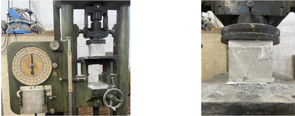
Figure 9: Compression Test Setup and failure
