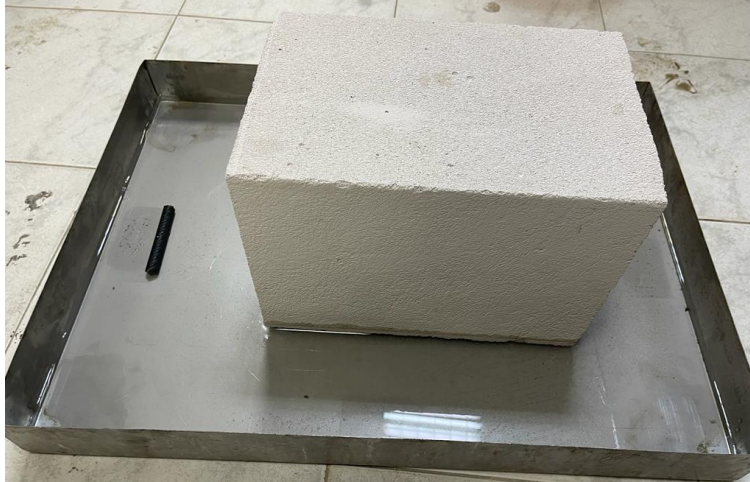
Figure 8: Initial Rate of Absorption Test Setup
