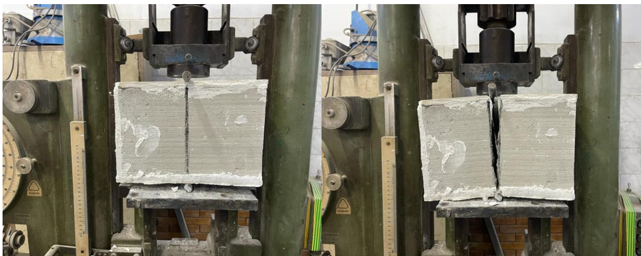
Figure 10: Splitting Tensile Strength Test Setup and Failure
