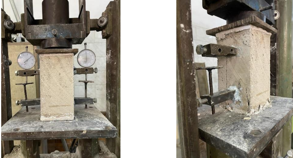
Figure 11: Modulus of Elasticity Test Setup and Failure
