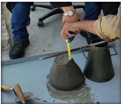
Figure 2. Shows the slump test.
