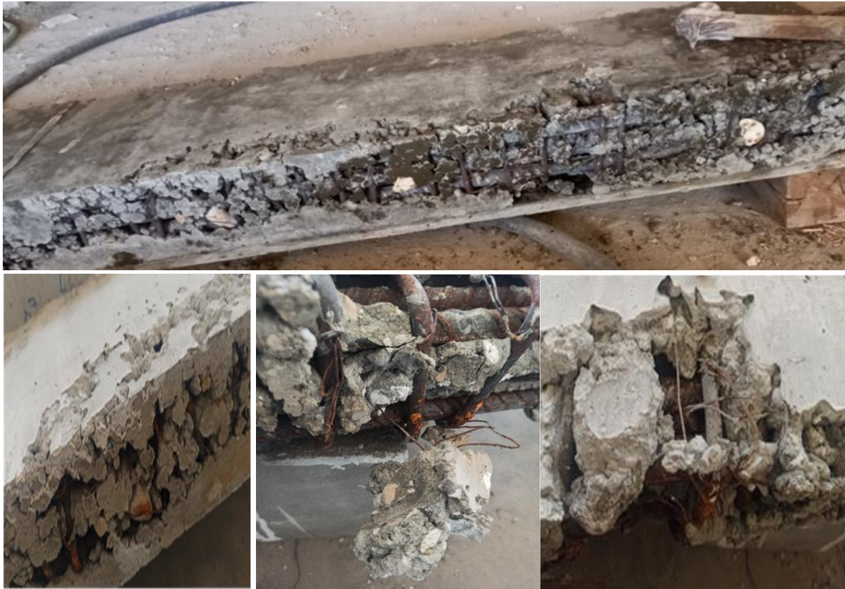
Fig.10: The surface finish and segregation on the bottom of the RC beam with NVC
