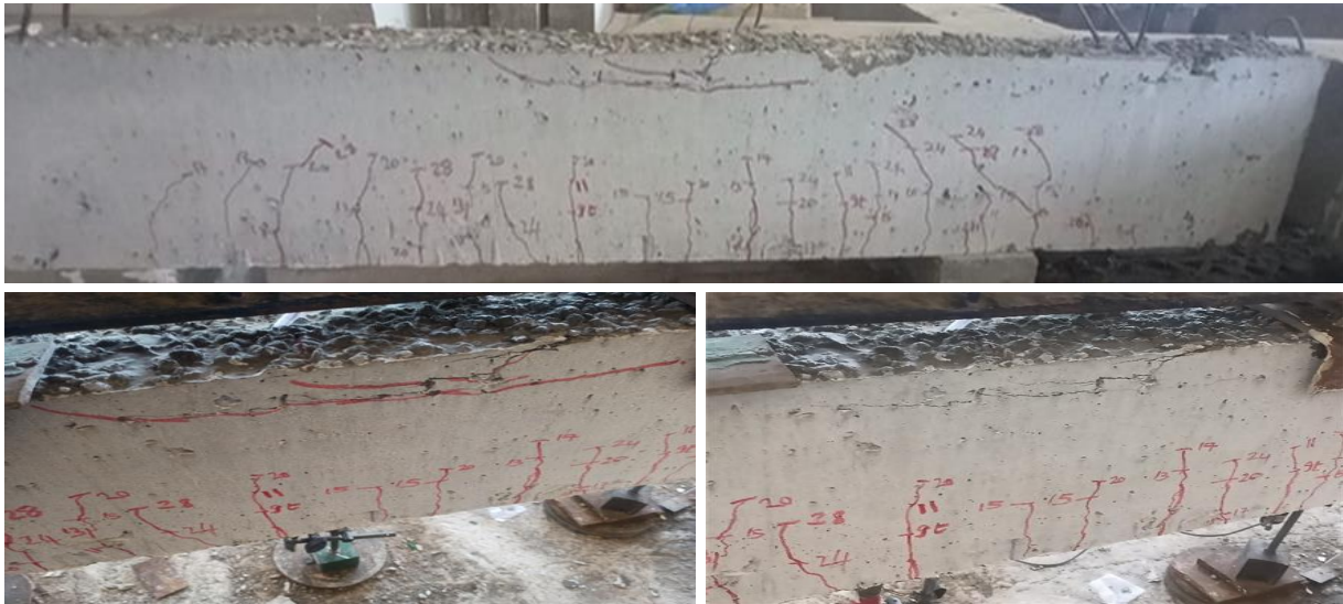
Fig.12: Crack pattern of beam SCC-B2 after failure
