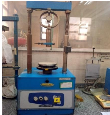
Figure 4. Determination of CBR by CBR apparatus
