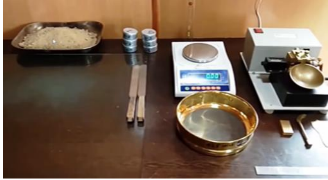
Figure 3. Determination of L.L and P.L by Casagrand apparatus.
