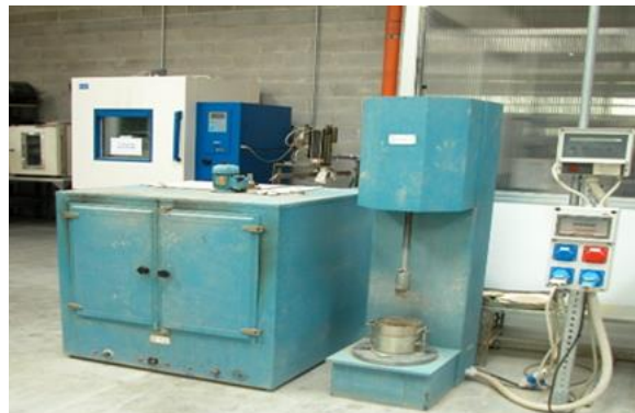
Figure 5. Determination of OMC and MDD with a proctor test.
