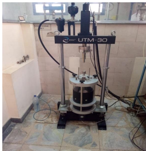
Figure 7. Repeated loading triaxial cell and soil specimen (universal test machine UTM).
