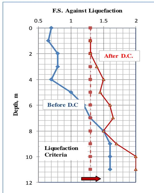
**Figure 8** Effect of Dynamic Compaction on the Soil Liquefaction Resistance
