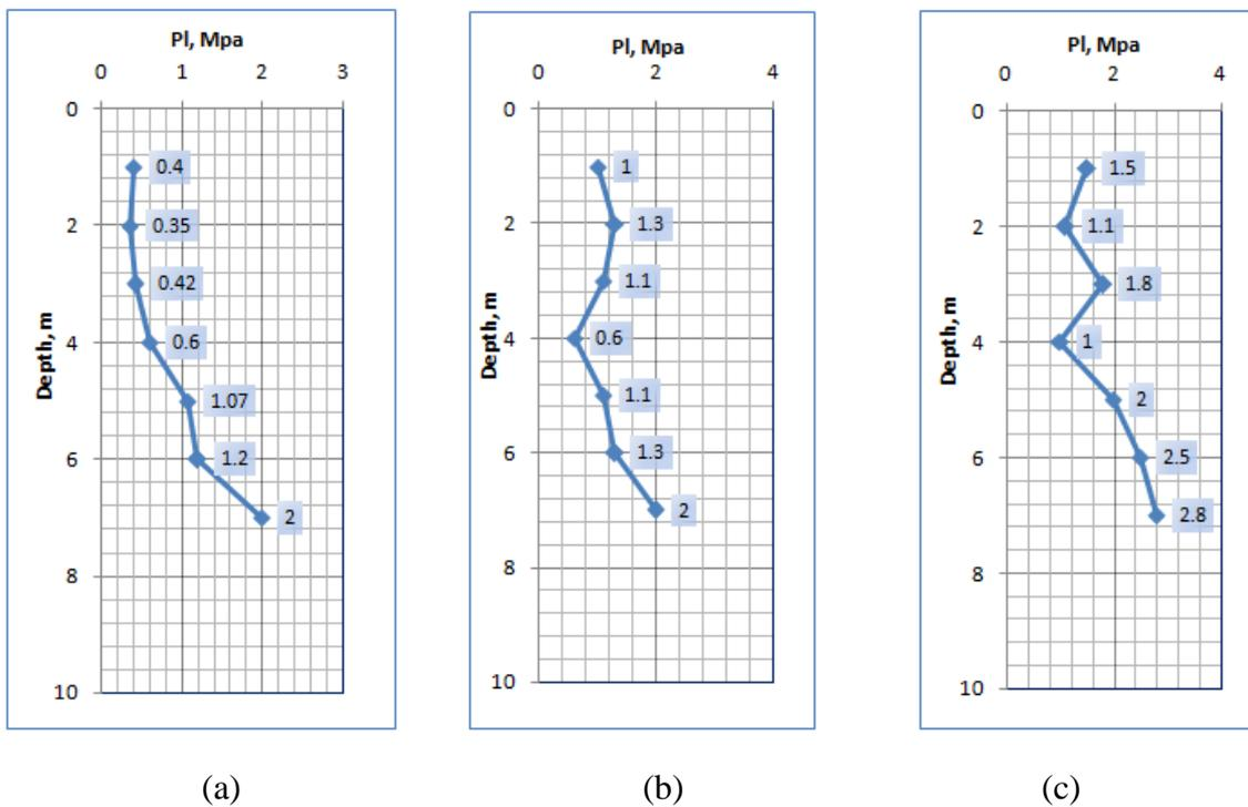
**Figure 5** PMT- Limit Pressure, PI Values a) Before D.C. b) after D.C Phase 1 c) After D.C. Phase 2
