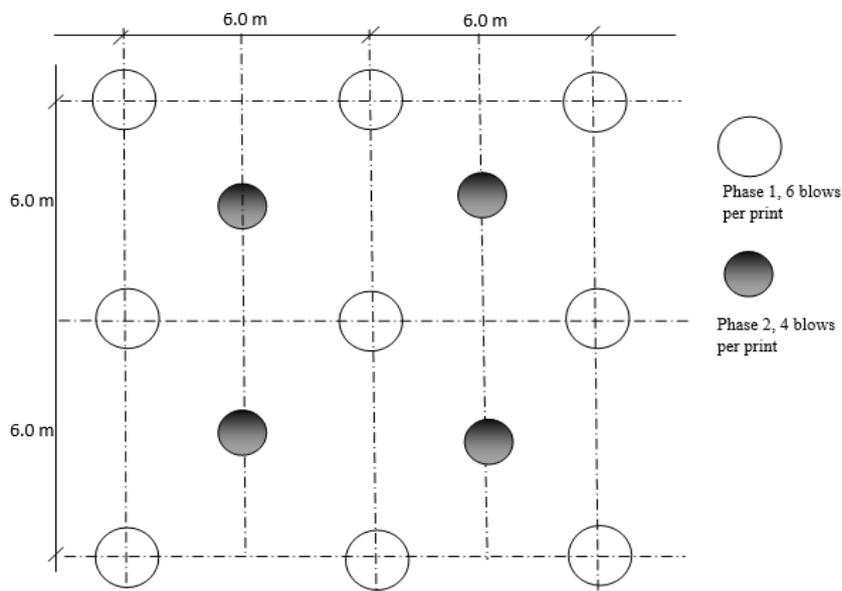
**Figure 4** Schematic layout of Dynamic compaction carried out at the site
