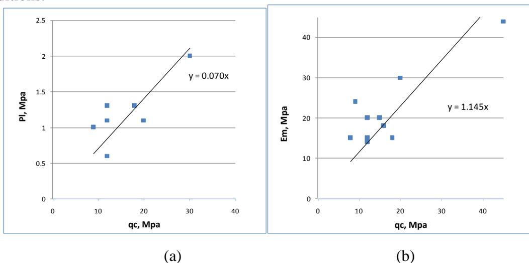
**Figure 9** Correlation between a) PMT-Pl and b) PMT-Em with CPT- $q_c$  values for sandy soils after Dynamic compaction
