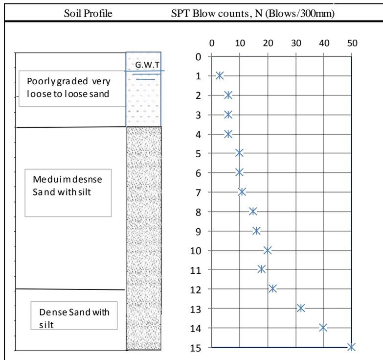
**Figure 2** Soil profile and SPT Results for the site under study
