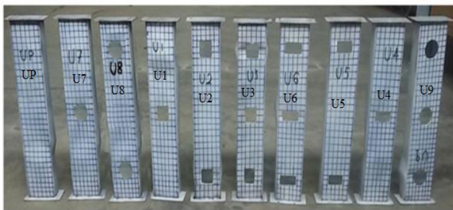
Figure (4) Steel columns with channel section by Sadjad A. Al-Jallad and Haitham Al Thairy, 2016
