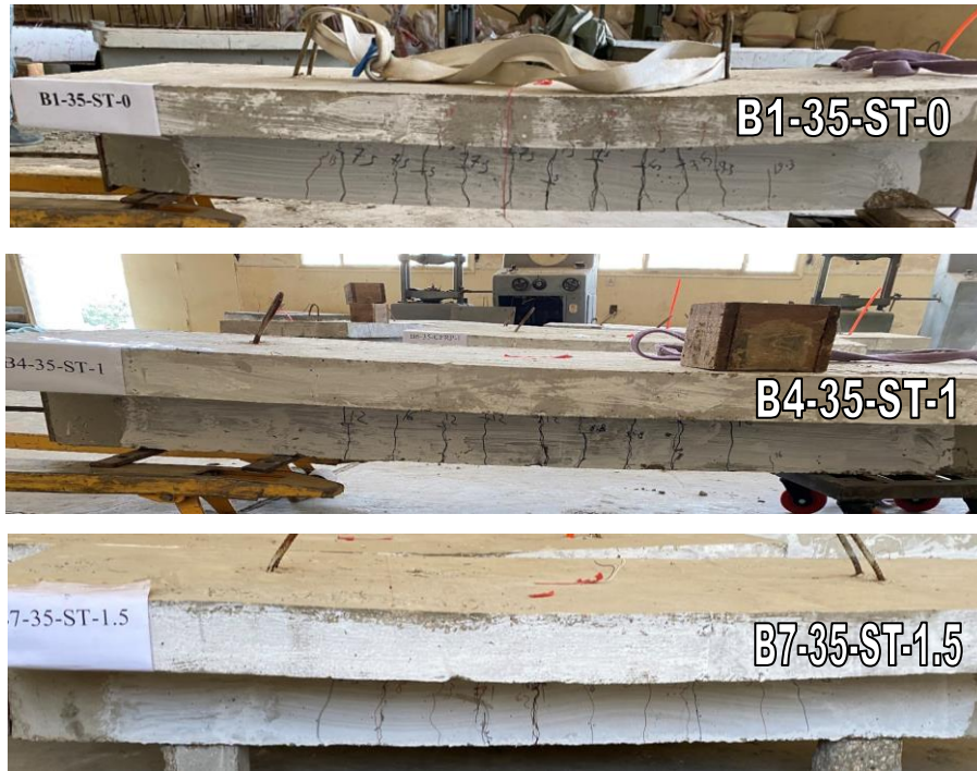
Figure (7). Cracks pattern of beams in Group 1
