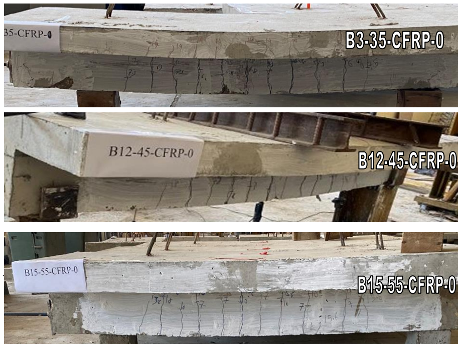
Figure (19). Cracks pattern of beam in Group4
