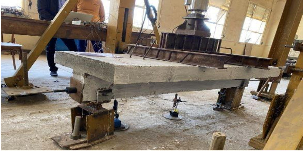
Figure (4). Test setup for flexural testing
