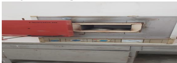
Figure (6): The crucible and the specimen were placed in the furnace
