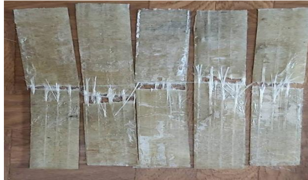
Figure (5): The specimen after the tensile test
