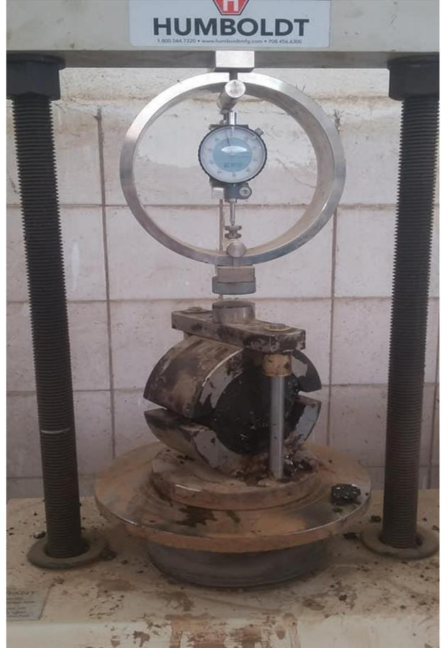
**Figure 4. Marshall Apparatus (HUMBOLDT) contents**
