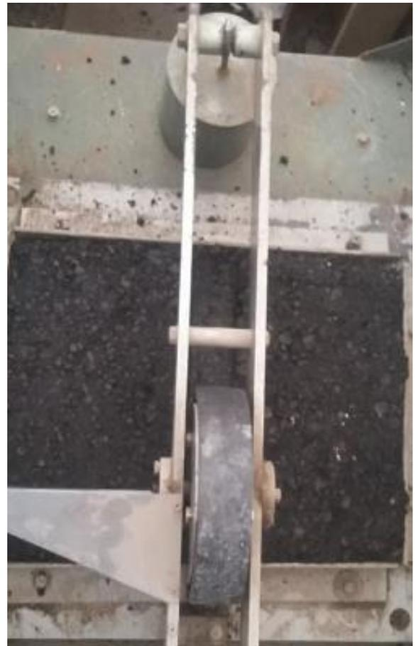
**Figure 7. Slab under wheel load**
