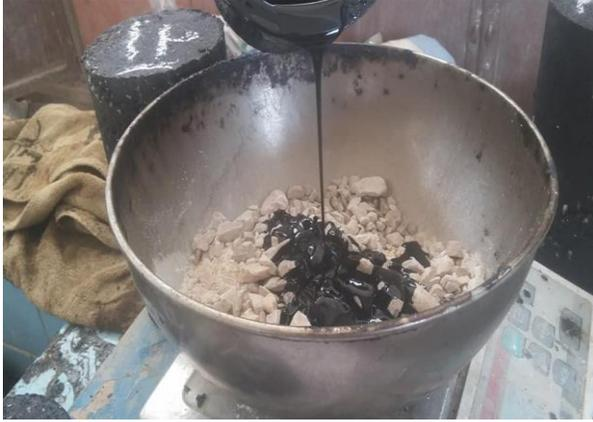
**Figure 2. Adding asphalt to aggregate**
