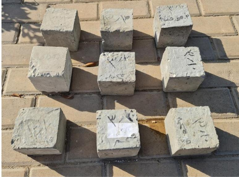
**Figure (3)** Un plastered concrete samples
