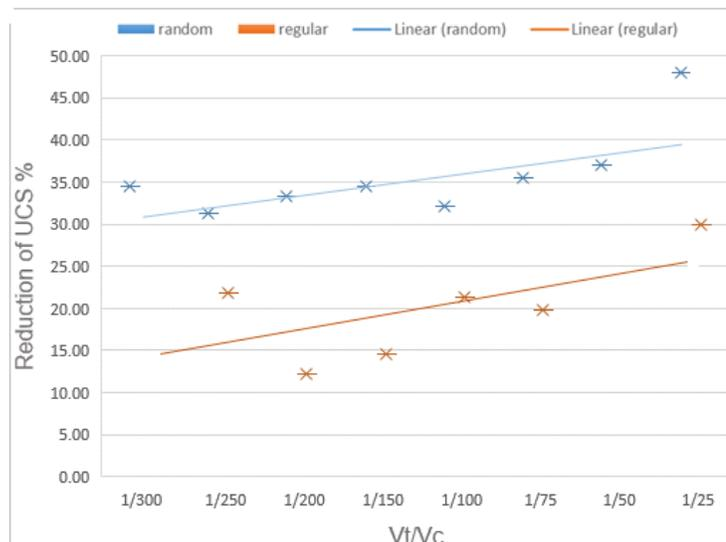
**Figure 5 Relation between  $V_c/V_t$  and the reduction ratio of UCS of rock with random and regular discontinuities**
