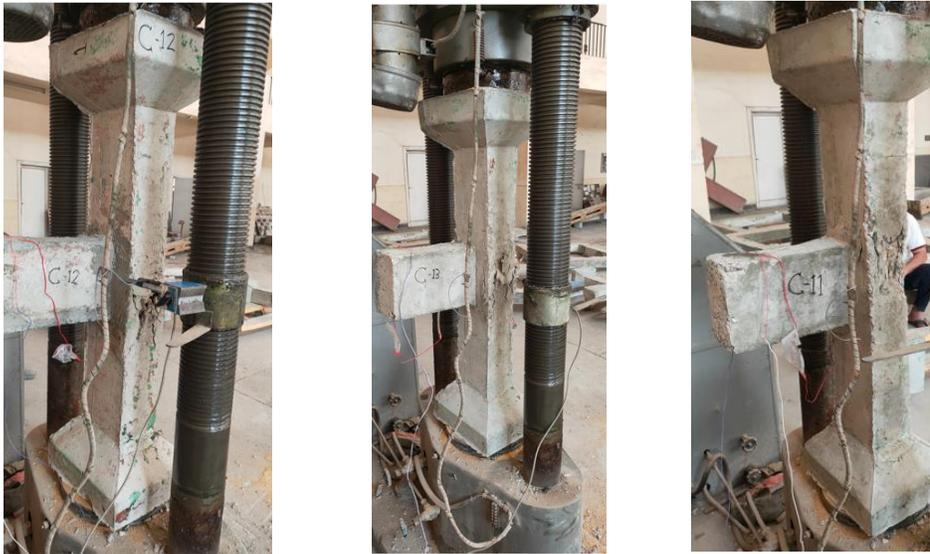
Figure 5 Cracks Pattern for All Columns
