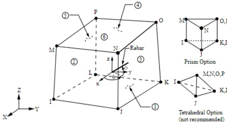
Figure 3. SOLID65 Homogeneous Structural Solid
