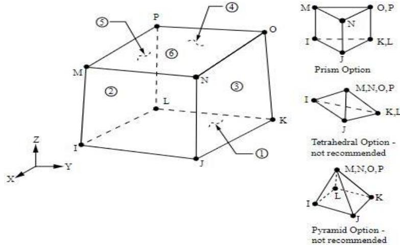
Figure 5. SOLID185 Homogeneous Structural Solid Geometry
