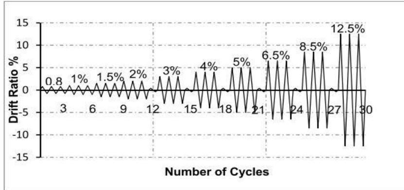
Figure 2- Seismic loading scheme
