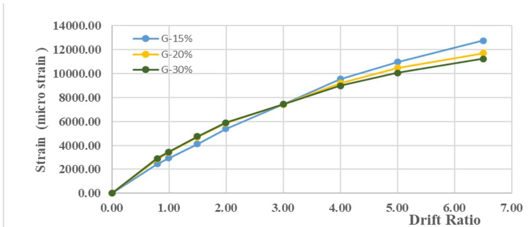
Figure 14. Maximum strain–drift ratio relationship for the longitudinal bars in Specimens.
