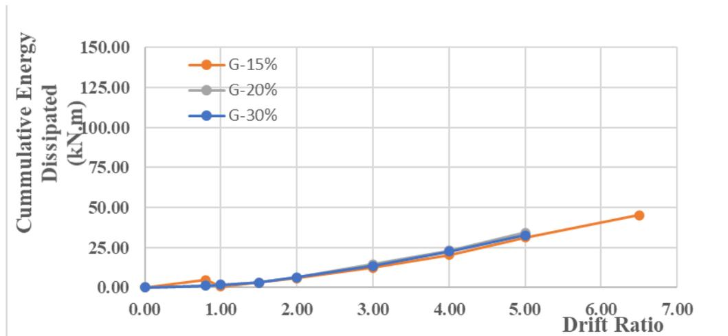
Figure 13. Cumulative energy dissipated
