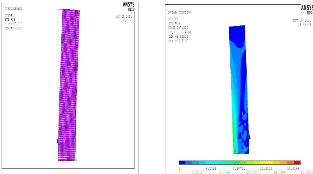
Figure 9. Displacement and Stress of column with 15% of axial load
