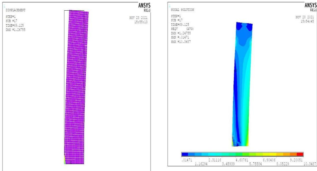
Figure 11. Displacement and Stress of column with 30% of axial load
