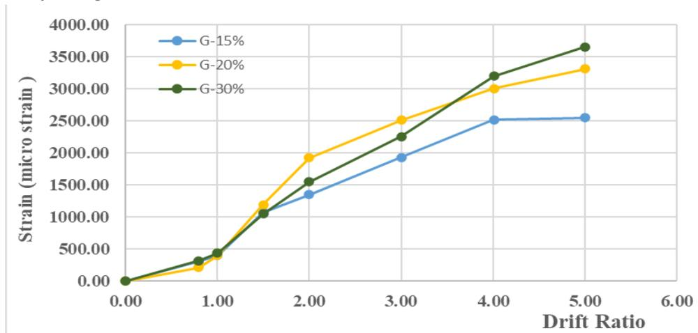
Figure 15. Maximum strain–drift ratio relationship for stirrups in Specimen.
