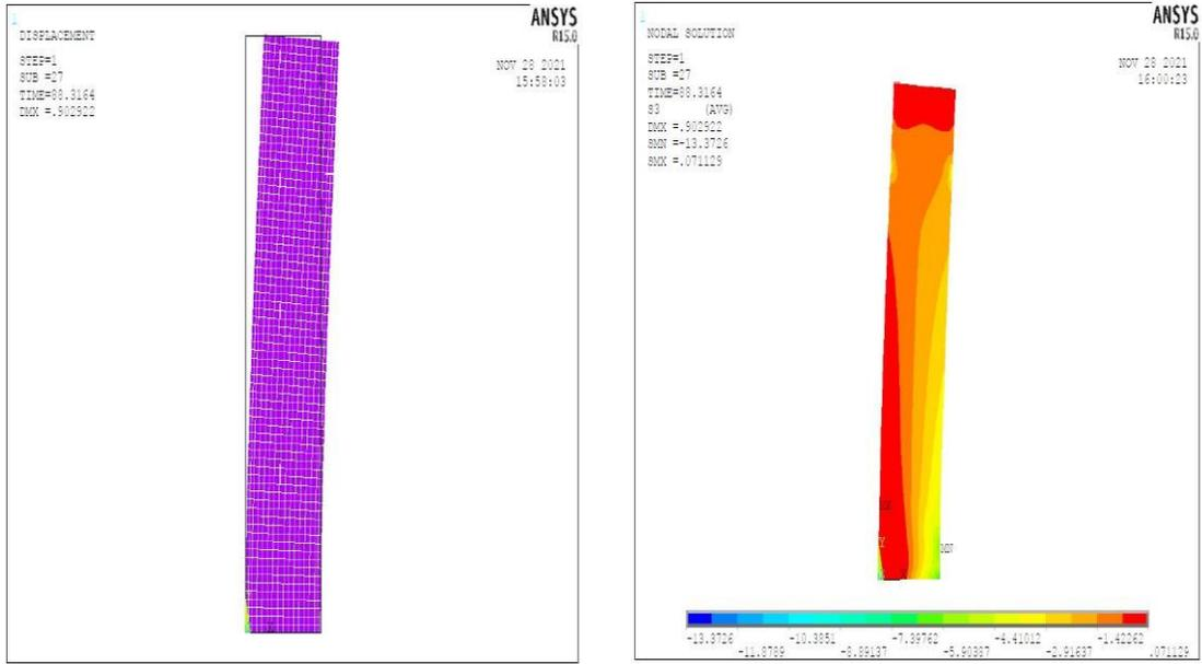
Figure 10. Displacement and Stress of column with 20% of axial load
