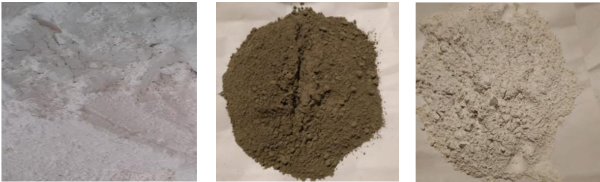
Fig. 1 The appearance of the two types of fillers: (a) Limestone dust; (b) Ordinary Portland cement; (c) Hydrated lime
