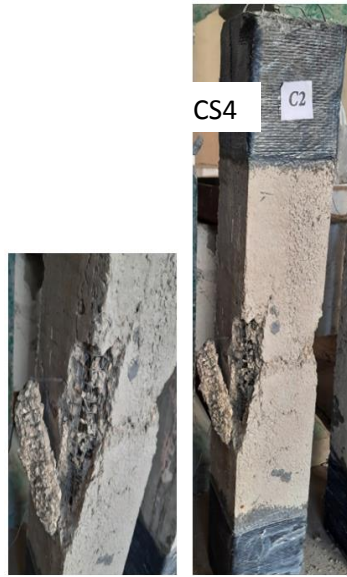
Figure 31 crack pattern of composite column (CS 4 ) confined with 2 layer of steel wire mesh.
