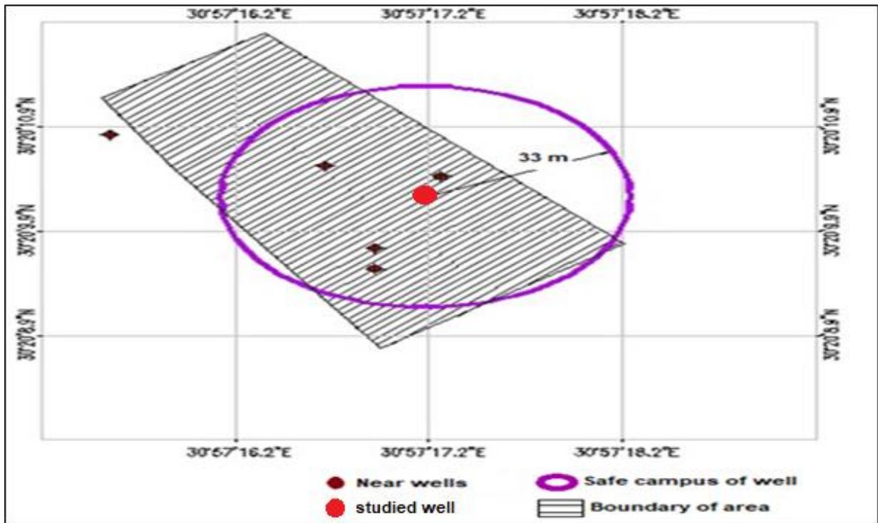
**Figure 17: The safe campus around the well according to the numerical model**
