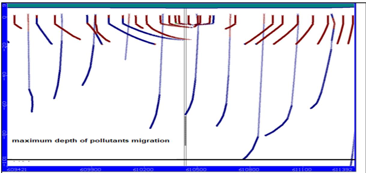
Figure 15: Cross-section for Path lines migration through aquifer layer
