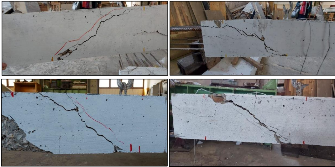
Fig. 3: Cracks at Failure of Slabs S1, S2, S5 & S6 respectively
