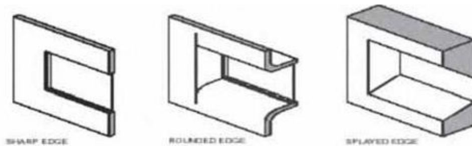
Figure no. (9): Chamfering window edges
