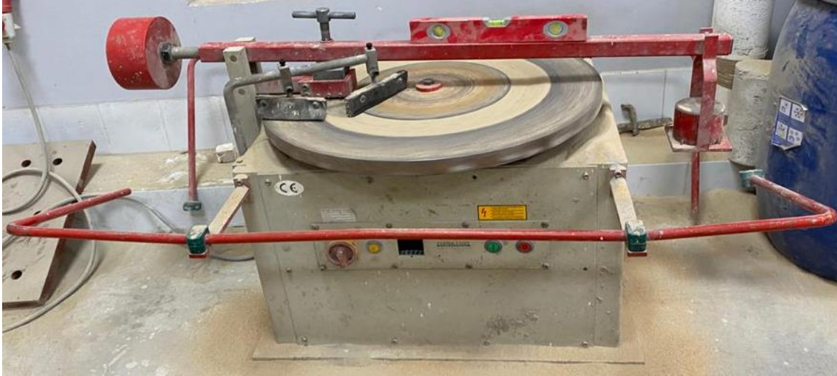
Figure 6: Typical specimen under abrasion testing
