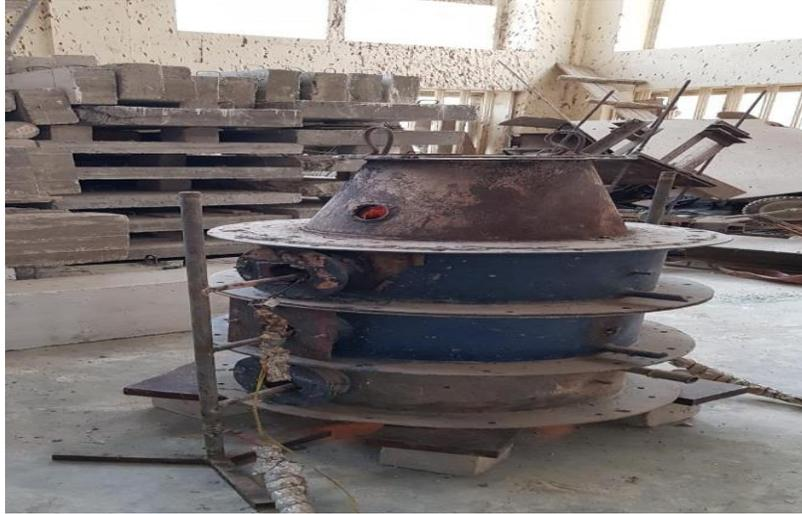
Fig. (2): An oven for burning samples.
