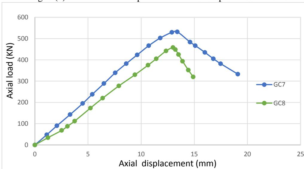
Fig. 6 (c): Load–vertical displacement relationship of GC7and GC8.
