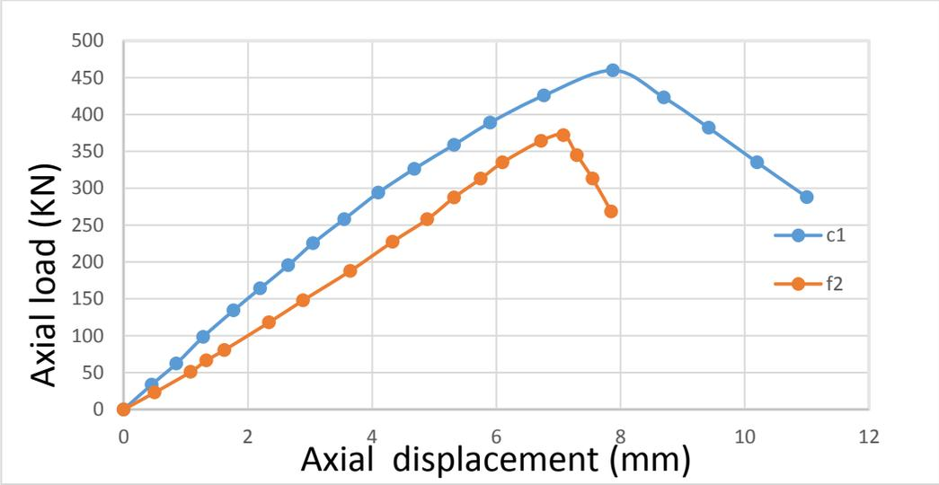
Fig. 5: Load–vertical displacement relationship of C1 and f2.
