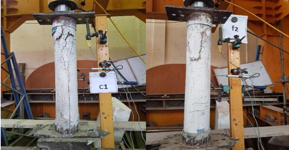
Fig. 3. Tested specimens of first group.
