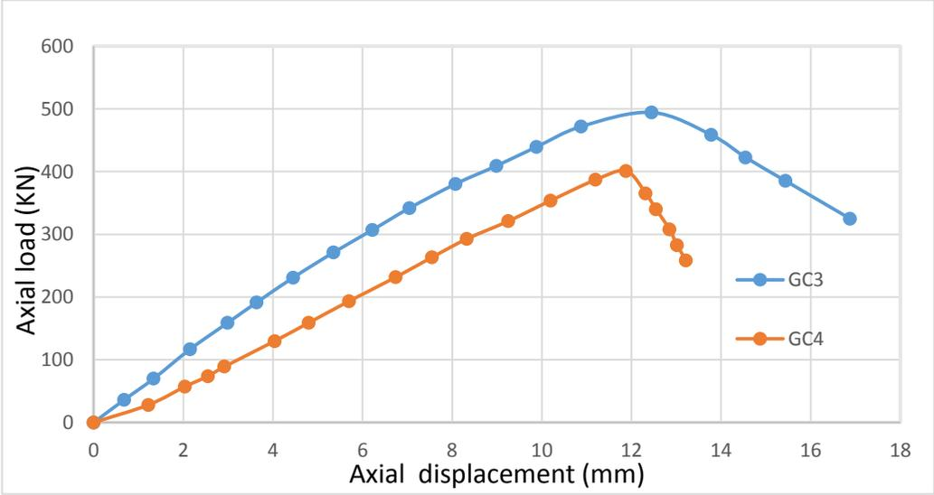
Fig. 6 (a): Load-vertical displacement relationship of GC3 and GC4.
