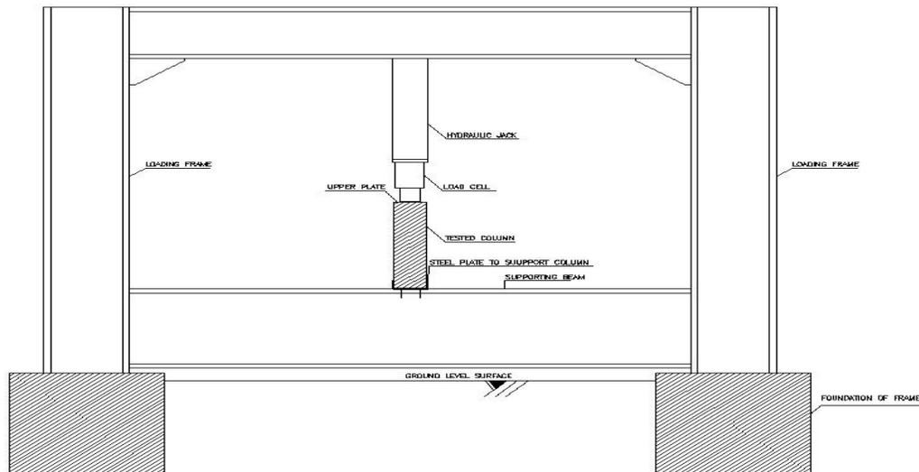
Fig. (3): Details of testing machine.
