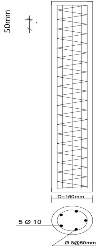
Fig. (1): Details of tested columns
