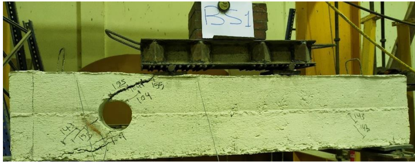
Fig. (4).Cracking Pattern for Beam (BS1).
