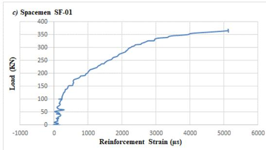
Fig. 7 The Relationship of Load and Reinforcement Strain for the tested specimens
