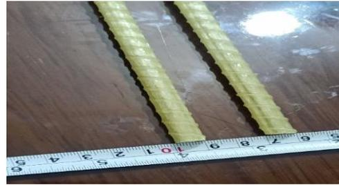
(b) Used GFRP bars with a diameter of 10
