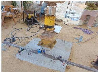
(b) Linear Variable Differential Transformers (LVDT's) Gauges positions
