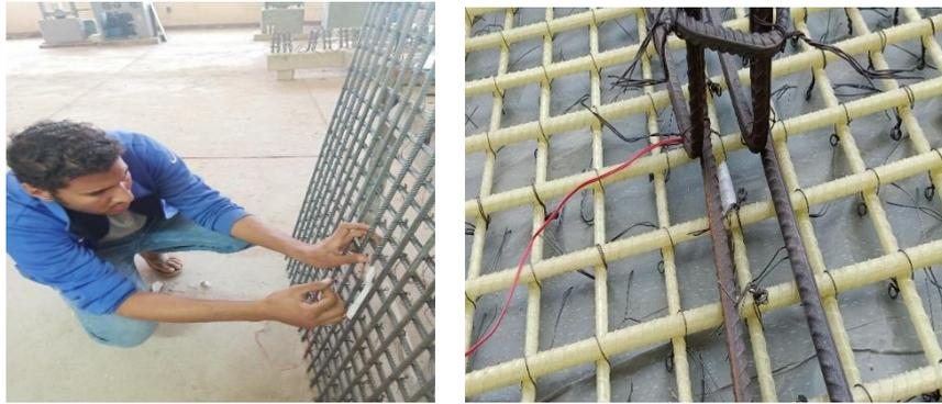
(a) Reinforcement electrical strain gauge location
