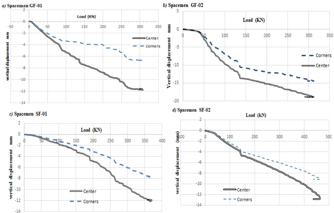
Fig. 5 The Relationship of Load and Vertical Displacement for the Tested specimens
