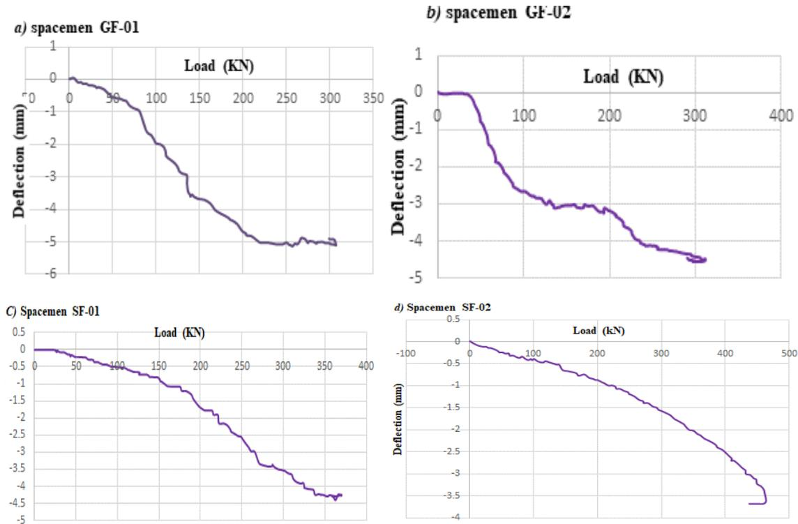
Fig. 6 The Relationship of Load and Deflection for the Tested specimens
