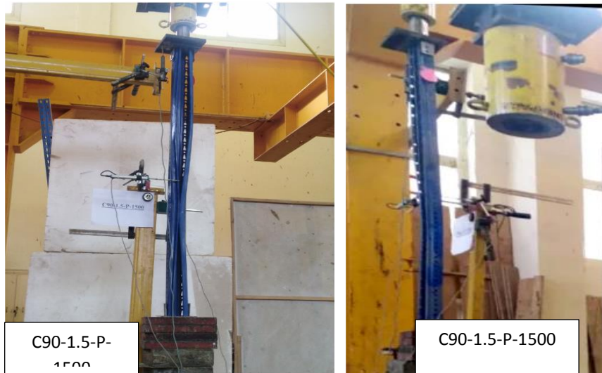
Figure 4. Buckling failure mode of C90-1.5-P-1500 specimen.
