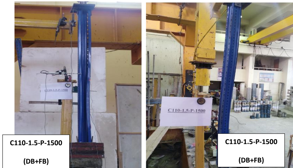
Figure 7. Buckling failure mode of C110-1.5-P-1500 specimen.
