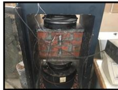
Figure 10. Failure mode of prisms under in-plan splitting tensile test with \theta = 0^\circ
