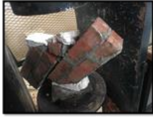
a. Prism constructed using mortar PW.
