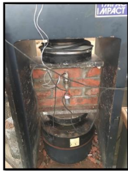
a. Prism constructed using mortar PW.
