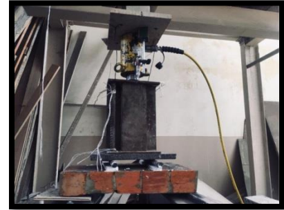
b. Prism constructed using mortar STWW.
