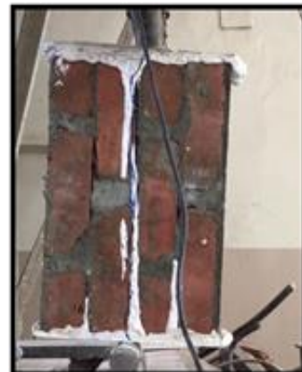
b. Prism constructed using mortar STWW. Figure.
