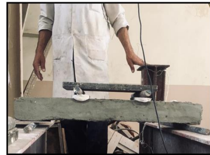
b. Prism constructed using mortar STWW.
