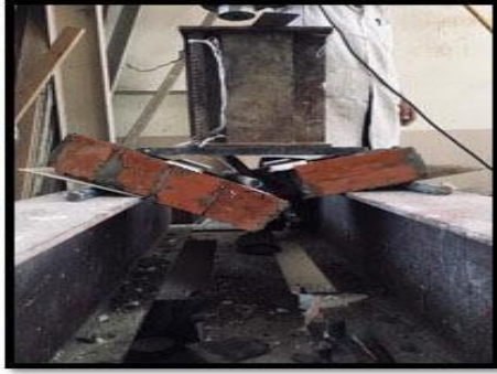
a. Prism constructed using mortar PW.
