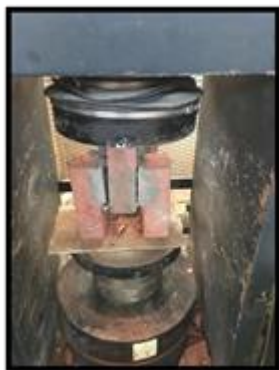
a. Prism constructed using mortar PW.
