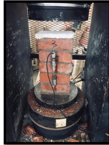
b. Prism constructed using mortar STWW.
