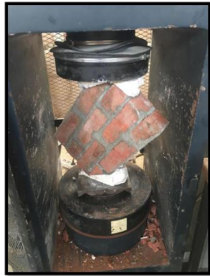
a. Prism constructed using mortar PW.
