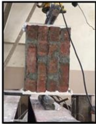
a. Prism constructed using mortar PW.
