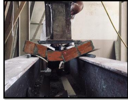
b. Prism constructed using mortar STWW.
