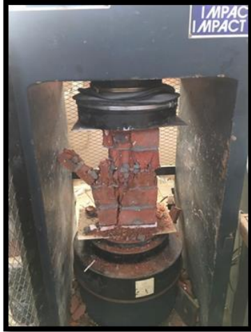
a. Prism constructed using mortar PW.
