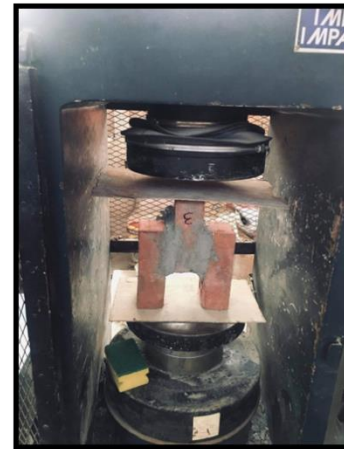
b. Prism constructed using mortar STWW.
