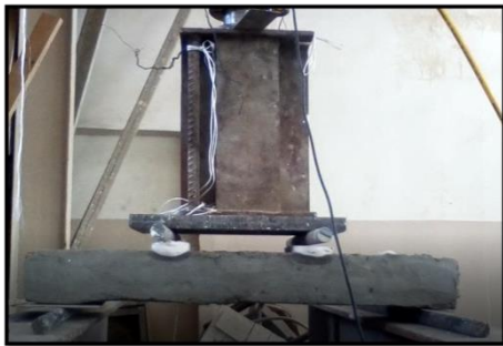
a. Prism constructed using mortar PW.
