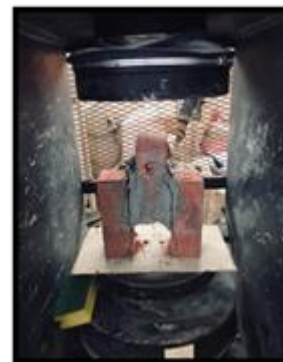
b. Prism constructed using mortar STWW.
