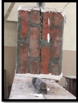
a. Prism constructed using mortar PW.
