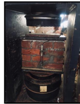
b. Prism constructed using mortar STWW.
