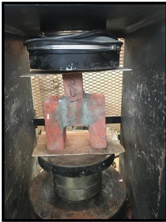
a. Prism constructed using mortar PW.
