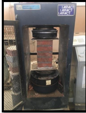
a. Prism constructed using mortar PW.
